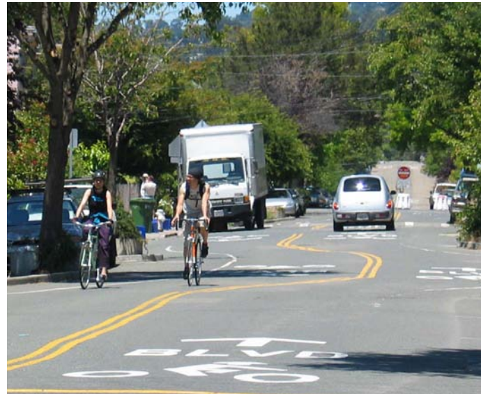
An example of a bicycle route where bicycles share the lane with traffic.
