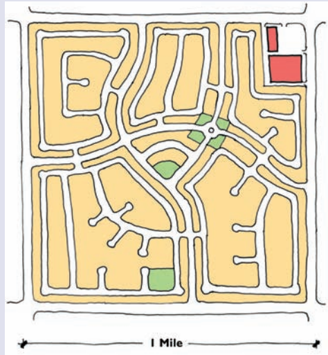
An example of a neighborhood designed for the automobile, with little thought given to creating pedestrian connectivity.
