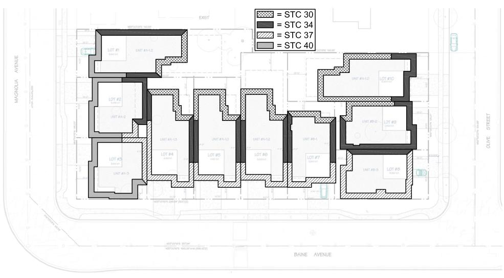
NOTE: STC RATINGS ARE FOR THE COMPLETE ASSEMBLY (E.G. GLASS, FRAME, AND OPERABLE SECTIONS) BASED ON TEST REPORTS FROM AN NVLAP ACCREDITED LAB.
