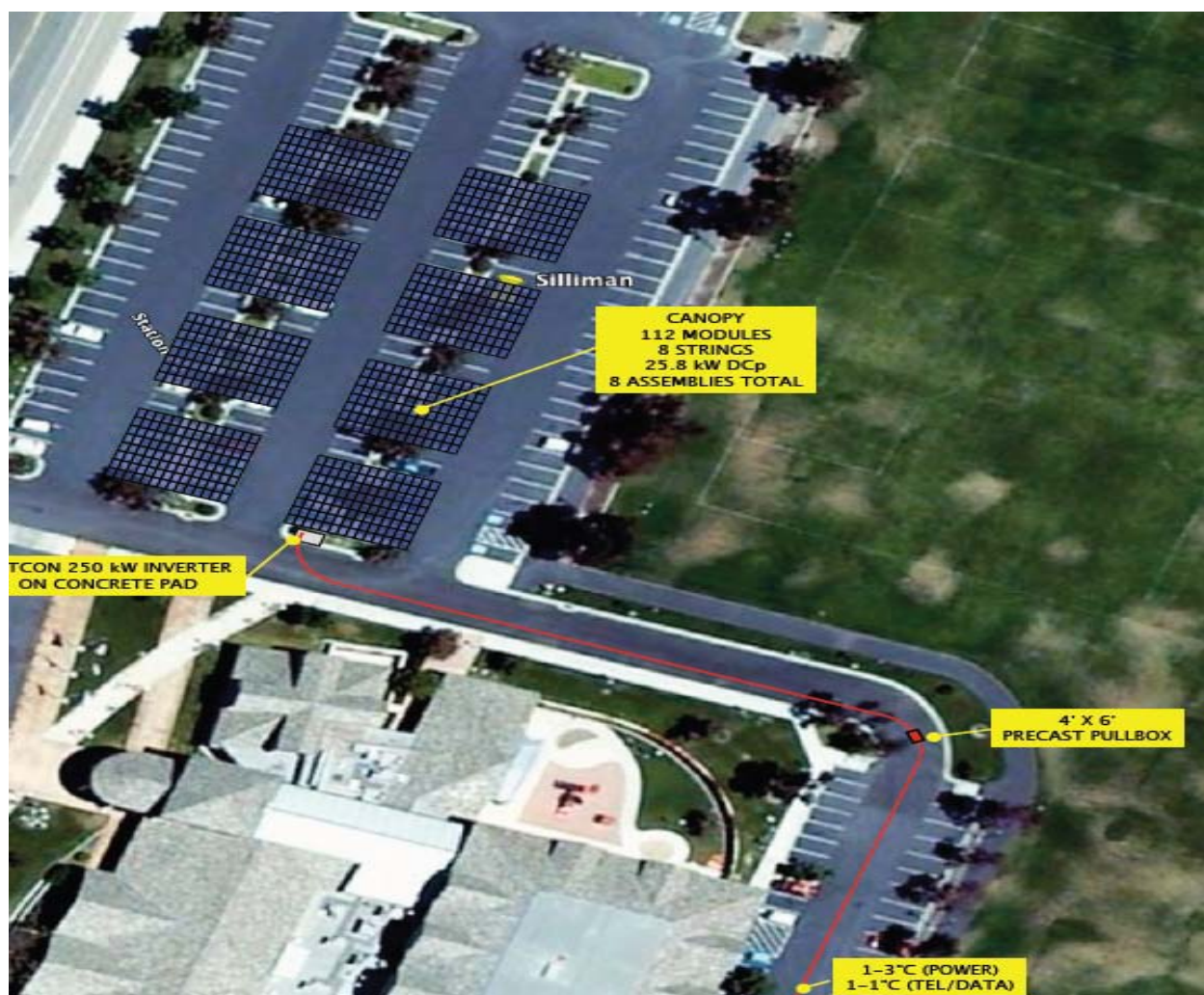
Figure 4.2 SAFAC Solar PV installation parking structure for illustrative purposes only. View - north parking lot carports- Red line is where trenching would occur for installation.
